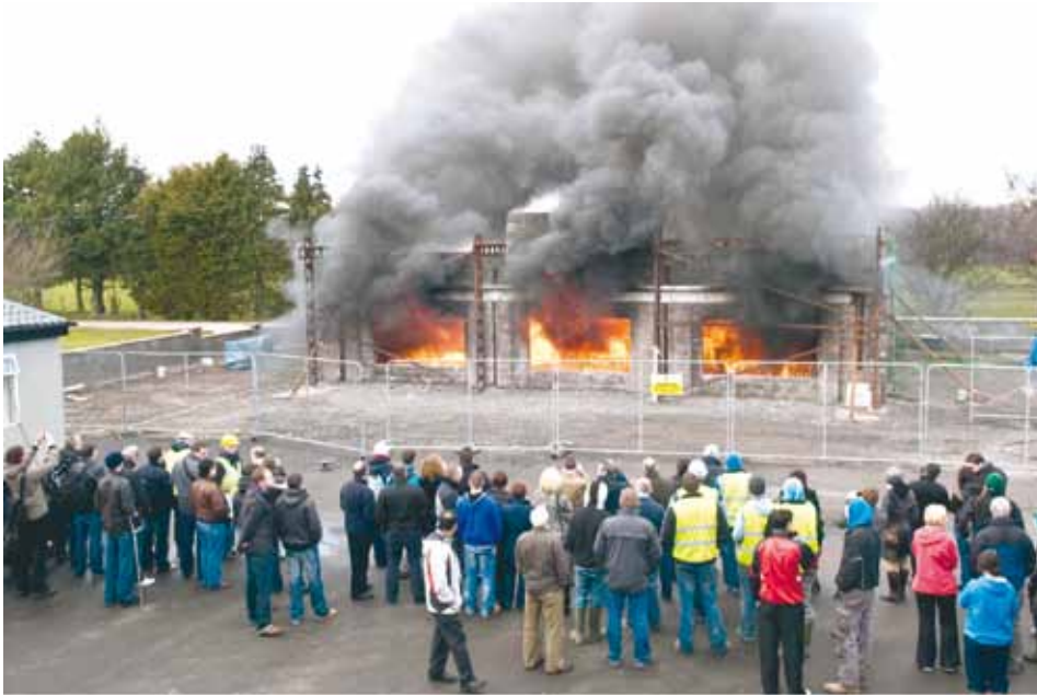
Unique Fire Test of Full Scale Compartment with long Cellular beams, FireSERT, Castledawson 27 th February, 2010.
