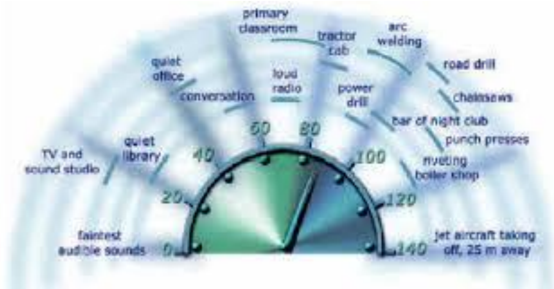
Fig 2 - 3dB increase can reduce exposure time by 1/2 (3dB increase doubles noise intensity at the ear)
