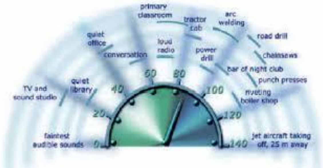
Fig 2 - 3dB increase can reduce exposure time by 1/2 (3dB increase doubles noise intensity at the ear)
