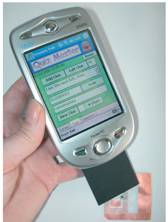
A handheld personal digital assistant (PDA) scanning a tag to find the next clue in an outdoor treasure hunt game
