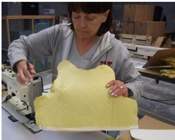
Building multi-layer Kevlar into 3 dimensional form
